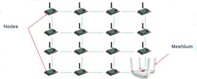
Figure 4: Waspote mesh network typology
