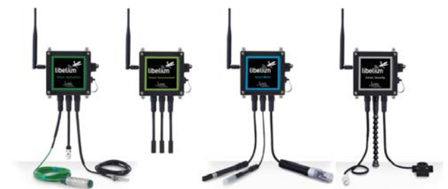
Figure 2: Libelium Smart Agriculture, Water, Environment, and Security Models used in UQSmart Campus initiative 2016. Images of models from Libelium webpage - http://www.libelium.com/products/plug-sense/models/ and a list of sensors being used at UQGatton from Libelium http://www.libelium.com/products/plug-sense/models/
