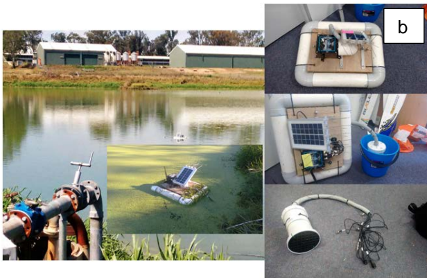
Figure 3a): Multisensor Mesh physical set up on farm; Figure 3b) Smart Water node on UQGatton Environmental Management lake – Lake Galletely
